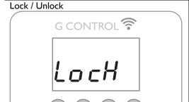
During any operation mode, it is possible to lock the keyboard by holding and simultaneously for 3 seconds. When the keyboard is locked, the message **Lock** will be displayed.
