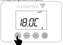
In manual mode, the unit will maintain the temperature set point and will ignore the pre-set program. SSH will maintain the selected temperature for the 24 hours of the day. Use this mode, when the same temperature is desired for every hour in the week.
