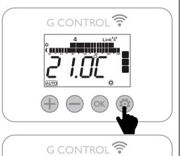
It is possible to modify the general settings. During any operation mode, press & release , the display shows the flashing temperature symbol F. and the RF symbol F.
