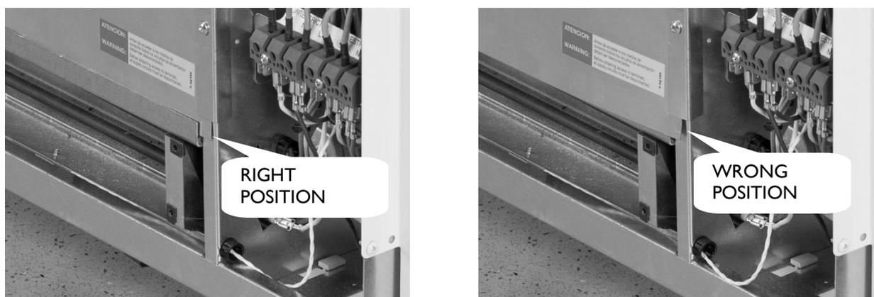
12. - Replace the front panel with screws. When replacing the exterior front panel, align the 2 plastic upper pegs on the heater with the holes in the exterior panel. Push the top up into place and push the bottom and fix the panel with the removed screws.
