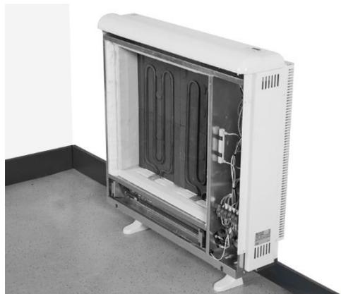
9. - Place the heating elements back into their original position. Place the second row of storage bricks with the flat side facing out and always on the heating elements supporting tabs.
