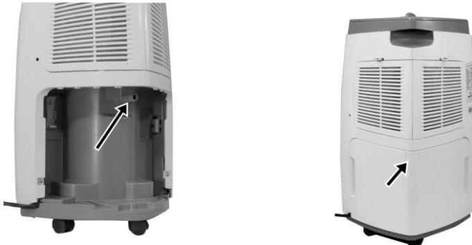
Use a hose with an internal diameter of 12mm (½"). Make sure that the hose runs downwards throughout its entire length, and has no kinks. Otherwise the drainage will not work.
