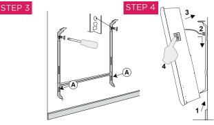
3. Place the wall bracket onto the bottom screws (A-A). Then fasten the wall bracket with the top screws.
