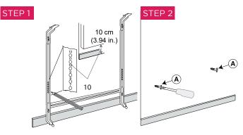
1. Use the wall bracket as a measuring device to place the heater on the wall.
