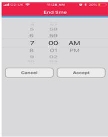
Make sure time zone 1 is highlighted in grey and the start time should be set as default to 00:00am. Leave that as it as you need to complete an instruction for every hour of the day for the cycle to be complete.
