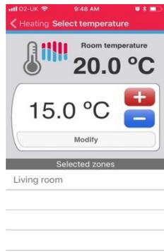
You can now turn the set point of the radiator up and down using your phone. If you click on the room on your phone, you can see the room temperature at the top right and the set point centrally in the white box. To adjust the temperature, use the red plus key or the blue minus key to adjust accordingly, then you must press modify to send the instruction to the radiator.
