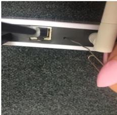
Now press the inset button on the back of the router using a paperclip or such like to put the gateway hub into pairing mode. This is just one short press.
