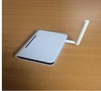
Open the box that contains the AeroFlow gateway hub. Thread the antenna into the back of the gateway hub. Plug the other end of the Ethernet cable into your internet router.
