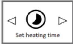
To program your radiator, press OK once to illuminate the screen, then ok again to access the parameters menu. You should now see 'programs'. Press 'OK here and you will see 'see' Press the arrow down button to see 'set heating times and press OK.
