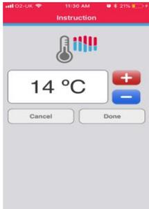
Now click in the 'instruction' box to select the desired temperature for this time frame. Again, most people don't want to heat the temperature too high during the evening, so we can select a relatively low temperature, for example 14 degrees. This means that the radiator will only come on if the room temperature falls to less than 14 degrees, and keep the room at this set point. Now press done.
