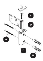
4- Insert the lower wall brackets (D) with the hook facing downwards into the bracket guide (C) (second position).
