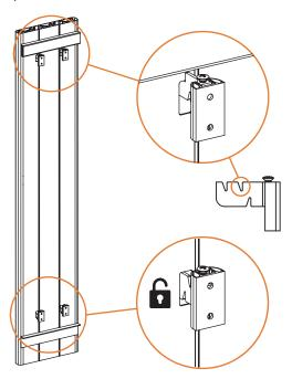
2- After inserting the wall plugs into the wall (B), install the bracket guides (C) on the wall by fixing them with the screws (A):
