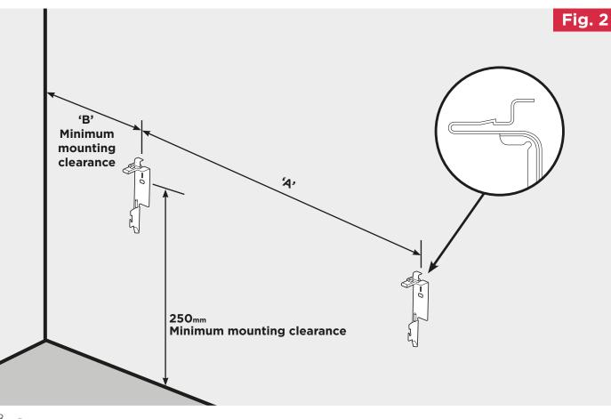
To mount the heater to the wall:
