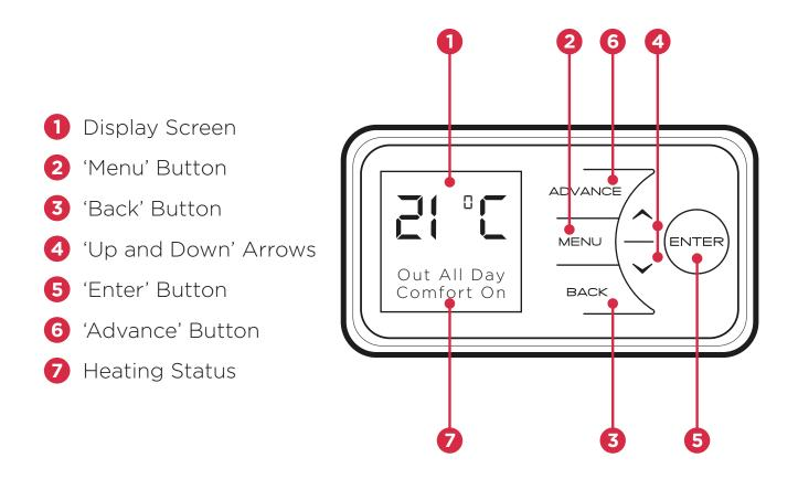
The heater is fitted with an adjustable thermostat enabling the room temperature to be controlled. The minimum room temperature is 7°C. The maximum temperature is set to 26°C by default however this can be increased to 32°C if required. A temperature of 21°C represents a normal room temperature.
