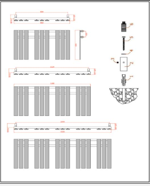
The radiator should not be mounted closer than 50mm below any overhanging surface i.ei shelf) and no lower than 100mm from the floor. Transfer the bracket drill position measurements to the
