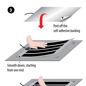
Apply pressure evenly over the full pad until it is completely flat on the mirror back
